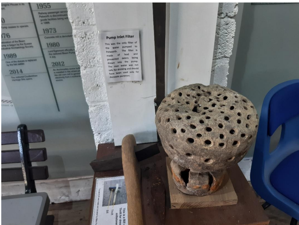
An inlet filter from Petworth House, used for filtering the river water pumped uphill from Coultershaw (July 2025).
